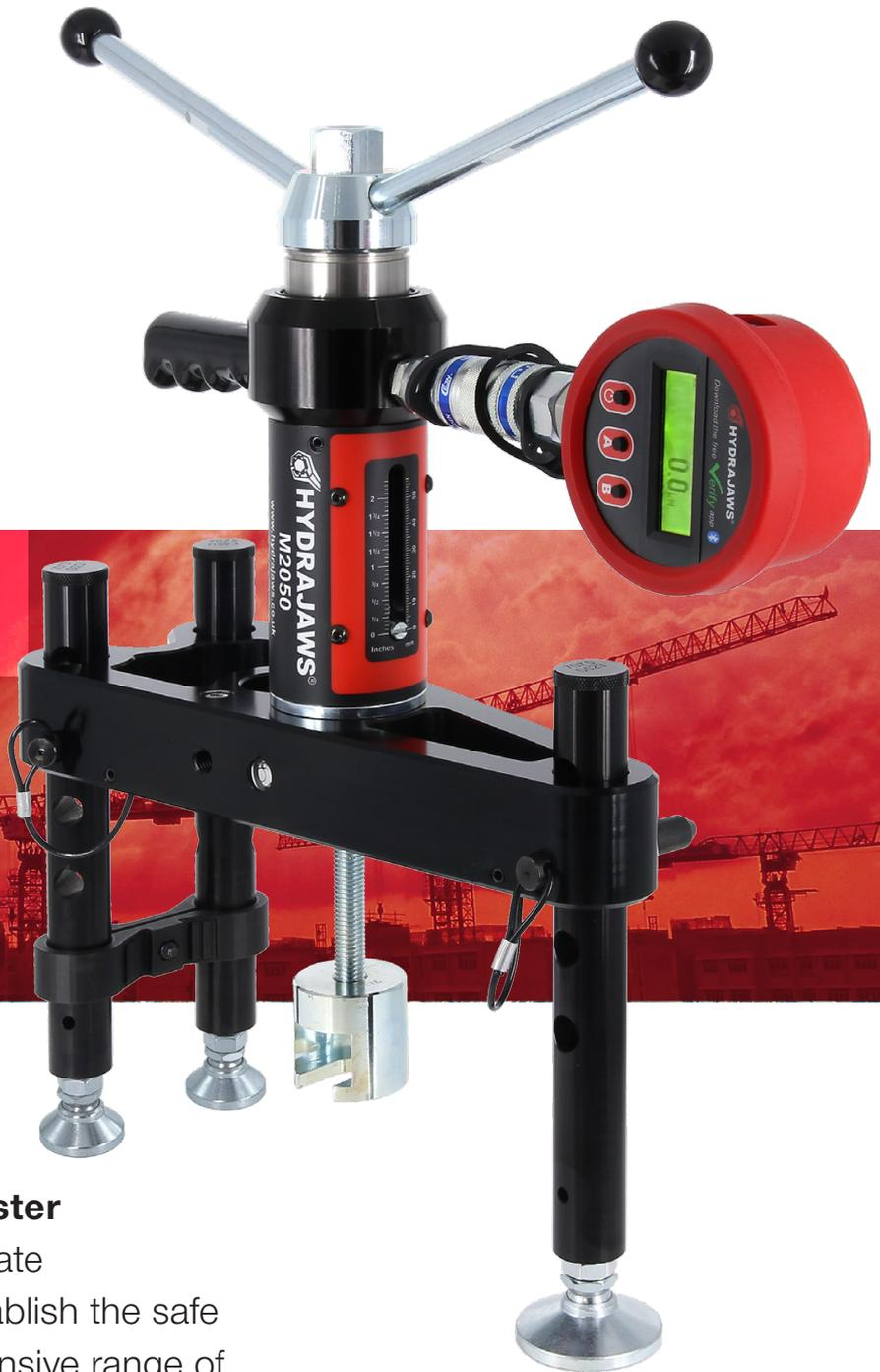
Extending the testing range to cover **0–50kN**, the **Hydrajaws M2050 PRO Tester** kit enables engineers to validate the correct installation or establish the safe working loads of a comprehensive range of anchors and fixings in line with BS 8539 up to a maximum tensile load of 50kN.
