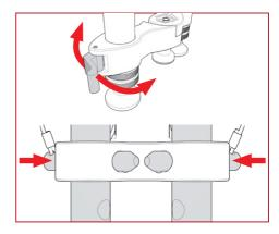
Loosen the thumbscrew of the Anti-Rotation Device.
