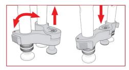
Unlock the two tabs to release the grip on the legs, rotate the legs until their holes are aligned and locked by their retaining pins, and then lock the leg brace tabs.
