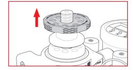
Unscrew and release the caps located at the top of the legs. These caps are magnetic and can be conveniently attached to the drop rod handwheel for safekeeping.
