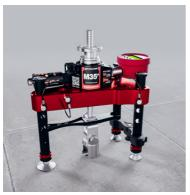
The optional Medium bridge can test up to **65kN** (14,613lbf), with a span of **210mm**.
