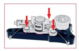
Take the two back legs and loosen the thumbscrew on the leg brace. Reposition the two pieces onto the appropriate lug. Tighten the thumbscrew. Then slide the legs into the larger bridge.
