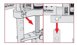
4. Then remove the two remaining leg pins and slide out the legs together.
