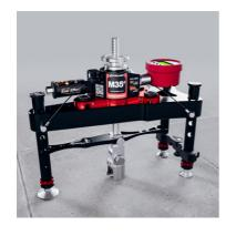
The optional Large bridge can span **310mm** and can test loads of up to **65kN (14,613lbf)**.
